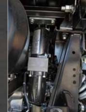
Electric hydraulic bed lift kit (left: dump switch / right: lift cylinder)
