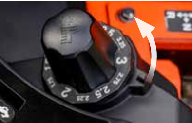
2 Use the dial to adjust the cutting height
