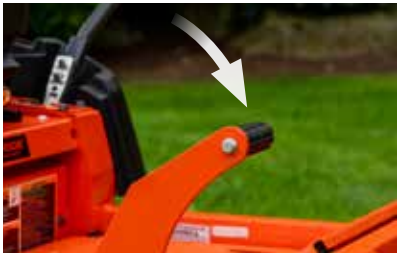
1 Push and release the pedal to raise the deck
